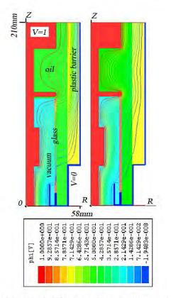
Fig. 3. Distribution of electric field (DC case to the left, AC to the right) in a shielded X-ray tube.
