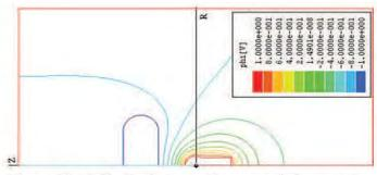
Figure 18. Field distribution with symmetrical connection, boundary open, f = 3.2, voltage phi = 1 V applied on the positive electrode (sphere mounted on a rod), voltage phi = -1 V applied on the negative electrode (a disk).
