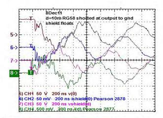
Figure 10. Short to ground, shield floats at distal end. Trace 5 (Chl) – voltage at proximal end; Trace 6 (Ch2) – current at distal end 0.5 A/div; Trace 7 (Ch3) – shield voltage at distal end; Trace 8 (Ch4) – current at distal end 0.5 A/div; Horizontal – 200 ns/div.
