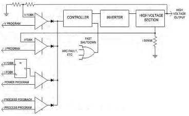
Fig. 3 Power Supply Control Loops
