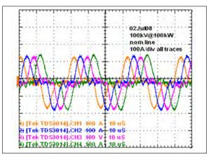
Fig. 6. π/4-phase-shifted primary windings currents (halved) at 100kV@100kW. Nominal line voltage 400 VAC.
