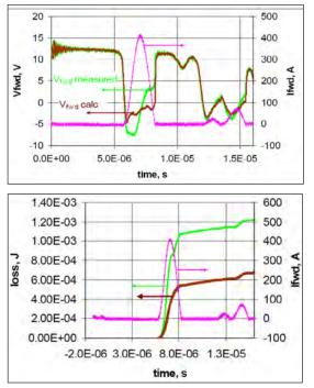
Fig. 9. FWD IXYS DSEI 2x61 losses. Plot a - green trace is measured signal; brown trace is Vfwd adjusted for inductive drop Ldlfwd/dt (diode assembly inductance assessed at 5nH). Green and brown curves plot b match their counterparts in plot a. Divider Fig. 7, Floating scope.
