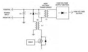
Fig. 4 Resonant Flyback/Forward Converter
