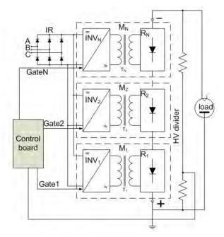
Fig. 1. HVPS block-diagram.
