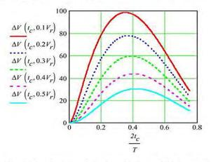
Fig. 24. Load voltage overshoot dependence on EOC timing  $t_c$  for  $V_T = 550$  V. Load voltage in fractions of  $V_T$  serves as parameter.
