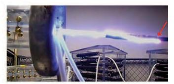
Figure 11. CUT#6. Photo of flashover. Positive polarity.
