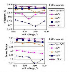
Fig. 13. Efficiency and power factor dependence on rail voltage for several charge voltages.
