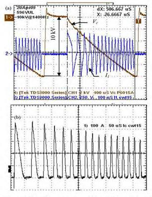
Fig. 11. Typical waveforms at high line. PRR = 1400 Hz in burst, charge time is 507  $\mu$ s. (a) Load capacitor voltage and primary winding current. (b) Collector current
