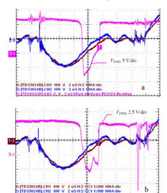
Fig. 11. Trace 3 - Forward drop of FWD IXYS DSEI 2x 61, two modules in parallel. a - high-bandwidth P6139A probe, b - differential probe. Both measurements taken with floating scope.
