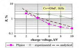
Fig. 10. Repeatability as a function of charge voltage-summary of PSpice and analytical calculations and experimental results.
