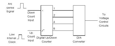
Fig. 6 Automatic Voltage Reduction Circuit
