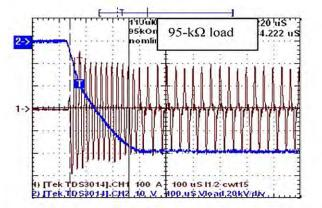
Fig. 10. Rise time across 95-k $\Omega$  load at nominal line. (Trace 2) Load voltage: 20 kV/div (measured by a specialty compensated voltage divider). (Trace 1) Primary current (halved): 100 A/div.
