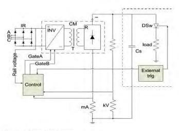
Fig. 1. Charger block diagram.
