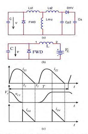
Fig. 21. (a) Full equivalent circuit (b) Reduced equivalent circuit. (c) Timing diagrams in normal operation (see Fig. 2 for notation).
