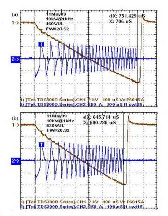
Fig. 12. Typical waveforms at 10  $\rm kV$  at 1000 Hz at (a) low and (b) nominal line.
