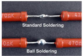
Ball soldering is a soldering technique frequently used in the high voltage industry. Large spherical balls of solder are used to make solder connections that are typically "at high voltage". The large diameter, smooth spherical shape of the solder connection helps to control the local E-Field, suppressing the generation of corona.
