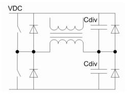
Fig. 2. Inverter with energy dosing capacitors
