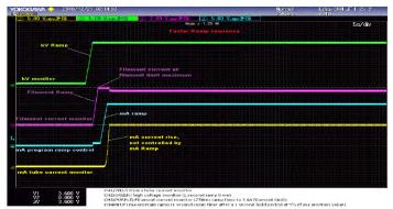
Figure 4: Filament and output currents during fast ramp.
