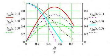
Fig. 25. Normalized inductor current and resonant cap voltage. Ut serves as a parameter.
