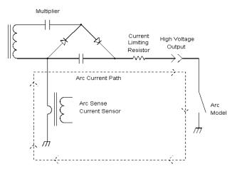
Fig. 3 Arc Sense Circuit
