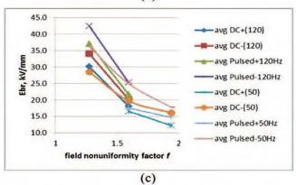
Figure 12. Test results (2011). (a) DC and pulsed test at PRR = 50 Hz, D = 20%. (b) DC and pulsed test at PRR = 120 Hz, D = 20%. (c) Dependence of the breakdown field  $E_{br}$  on field nonuniformity factor f. c is constructed using the data in a and b (note the uniformity of the data series legends in a, b, and c).
