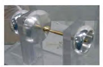
Figure 3. Sphere-to-plane spark gap.
