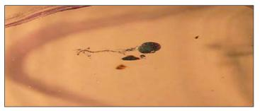
Figure 2: Magnified arcing area on the glass, showing a damaged tube wall.
