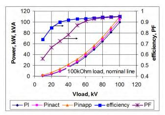
Fig. 11. Apparent, Pinapp, and active input power, Pinact, load power, PI, efficiency and PF at nominal line for  $100k\Omega$  load.
