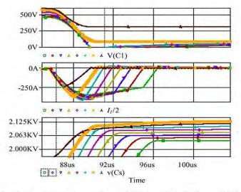
Fig. 7. Programmed charge voltage 2 kV.  $V_{\rm T} = 460$  V, 480 V, ..., 600 V.  $C_{\rm S} = 200$  nF. Primary current  $I_{\rm 1}$  is halved. Curves corresponding to largest overshoot are in thicker lines.
