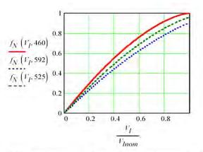
Fig. 3. ZCC curves for low (460 V), high (592 V), and nominal (525 V) dc rail voltages.  $V_{\rm inom}$  is nominal load voltage.
