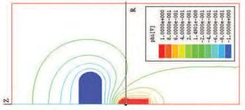
Figure 15. Field distribution with symmetrical connection, grounded boundary shown by red line. The positive electrode (a sphere mounted on a rod), shown in red, is held at potential phi = 1 V. The negative electrode (a disk), shown in blue, is held at phi = -1 V. Gap = 15 mm, field nonuniformity factor f = 2.8.
