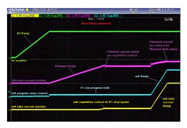
As you can see above in the waveform above, at the completion of the kV ramp the mA program steps to 5% of the programmed mA value. At the same time the filament slowly ramps up allowing mA regulation to take control. After mA regulation is in control and stabilizes, the mA ramps to the final program value with no over shoot. Note the filament current never goes to the maximum filament limit set point of 3.6A.
