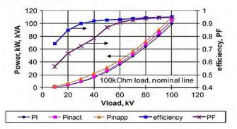
Fig. 11. Apparent (Pinapp) and active (Pinact) input powers, load power (PI), efficiency, and PF at nominal line for 100-k $\Omega$  load.
