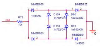
Fig. 7. Bridge formed by fast diodes around a Zener diode works equally well for measurement of positive and negative low voltages in wide dynamic range. Circuit excited by source V1 Fig. 2.
