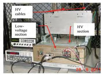
Figure 1. High-voltage power supply (HVPS) with unshielded polyethylene cables.
