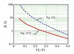
Fig. 9. Repeatability as a function of charge voltage,  $C_{\rm S}=200$  nF, C1 = C2 = 2  $\mu{\rm F},$  worst case.
