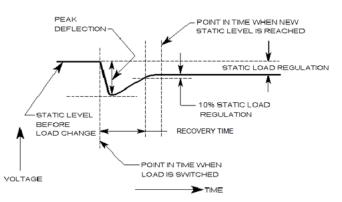
The voltage recovery waveform time period and overall shape (under damped, over damped or critically damped) are dependent upon the parameters outlined above in addition to the compensation characteristics of both the voltage and current loops of the power supply.
