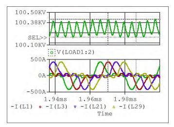
Fig. 8. HVPS circuit simulation. High line 580V. ripple 0.223% p-p. PF=0.943. Experimental PF= 0.946 (see Figure 11).
