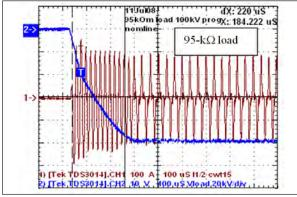
Fig. 10. Risetime across  $95k\Omega$  load at nominal line. Trace 2 – load voltage, 20kV/div; trace 1 – primary current (halved), 100 A/div.
