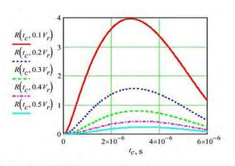
Fig. 8. Repeatability R % versus  $t_c$ , with load voltage  $V_L$  as a parameter (in fractions of the rail voltage, both reflected to the same side of HV transformer). Nominal load voltage (10 kV) is  $V_L \approx V_r/2$  for low line ( $V_r = 460$  V at primary side).  $C_s = 200$  nF, C1 = C2 = 2  $\mu$ F. Compare to Fig. 7.
