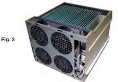
These test loads use an array of active MOSFET transistors. The transistors can be programmed to offer an infinite range of load configurations within the PFE's capabilities. In addition, highly compact Test Loads can be achieved. These modern Test Loads do come at a premium price though. However, their small size can offer a massive reduction in the size of the cabinets used for just the Test Load. Indeed, modern PFE's can
