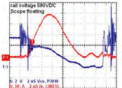
Fig. 3. Measurement of collectoremitter voltage Vce of CM300DC-24NFM Powerex IGBT using circuit Fig. 2. TDS 3024B scope is floating. In this and further plots, waveform notes carry scale information and types of probes used.
