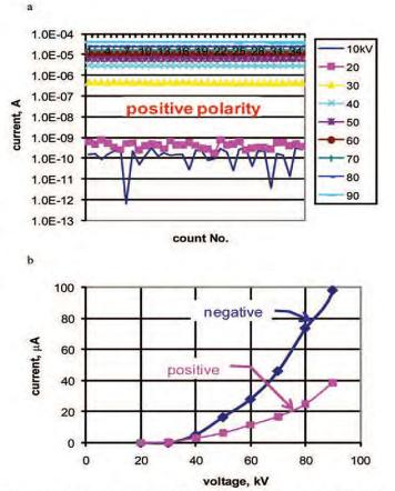
Figure 4. Leakage current (LC) for CUT#1 (flush cut, no shrink tube). a) LC dependence on time (count number) at positive polarity; b) LC as a function of applied voltage at positive and negative polarity.
