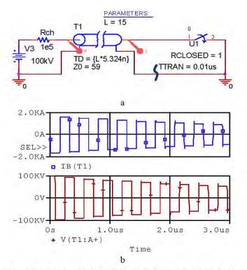
Figure 1. a - PSpice model of 15-m 2042 cable discharge on short circuit. Switch closing/transition time, TTRAN, is a PSpice parameter, it is much shorter than cable electrical length. b – timing diagrams. Current amplitude is V/Z.
