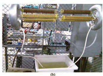
Figure 4. HV layout. (a) Shielded HV cables (partially visible). The load is supported by two HV dividers, HVD100 [12], allowing measurement of the voltage between the poles and ground. (b) Unshielded polyethylene cables. A resistive load shortens the voltage impulse fall time.
