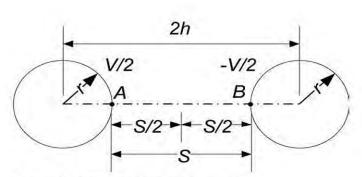
Figure 13. Sphere-to-sphere gap geometry.
