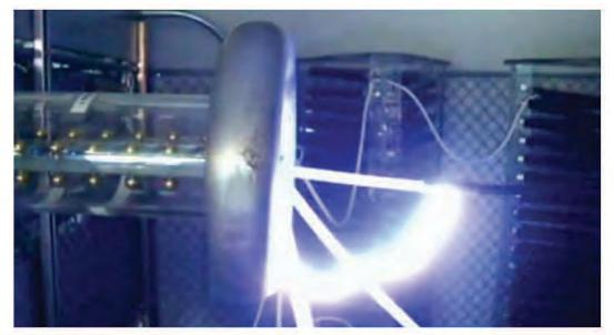
Figure 9. CUT#4. Photo of flashover. Positive polarity.
