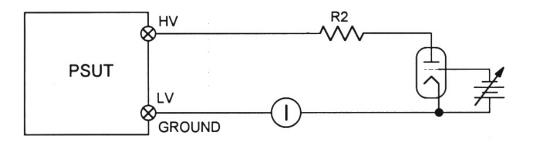
Figure 4. Electron Tube Switch
