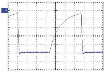
Figure 2. Typical output of the negative pole (-75 kV), with shielded cables. Load resistance = 83.5 M $\Omega$ . Pulse repetition rate = 15 Hz. Vertical scale 15 kV/div, with zero indicated by  $1 \rightarrow$ ; horizontal scale 10 ms/div.
