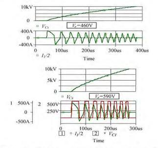
Fig. 6. PSpice simulation for 460 V and 590 V dc rail voltage. Parameters correspond to those of physical object (leakage inductance is L = 3.3 mH, reflected to secondary;  $C1 = C2 = 2 \ \mu F$  is resonant capacitor,  $C_s = 200 \ nF$  is the storage capacitance). Primary current  $I_1$  is halved.
