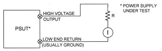
Figure 2. Constant Load Test Set Up
