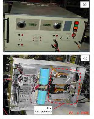
Fig. 5. Charger (a) front view and (b) bottom section.
