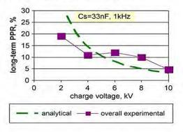
Fig. 20. PPR at low-capacitance charge.
