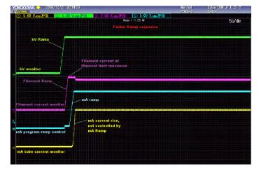
As you can see in the waveform graph the faster ramp sequence does not allow enough time for the X-Ray tube filament to achieve the required temperature for emission current before the mA ramp starts. The causes the filament current to ramp to the maximum filament limit and stay at that level for several seconds while the filament reaches required temperature for the requested emission current. The mA current rise is not controlled by the mA ramp and hence may have a slight over shoot.
