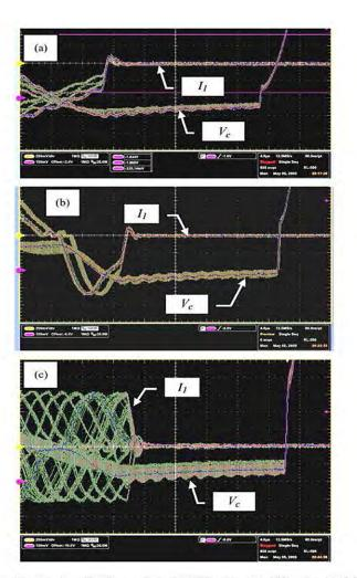
Fig. 15. Overlay of 80 frames ( $V_c$ -100 V/div,  $I_1$ -100 Å/div) for: (a) high line, 2 kV at 1 kHz; (b) nominal line, 6 kV at 1 kHz; and (c) high line, 10 kV at 1 kHz. Horizontal 4  $\mu$ s/div.
