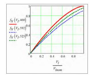
Fig. 3. ZCC curves for low (460V), high (592 V) and nominal (525V) DC rail voltages. VInom is nominal load voltage.
