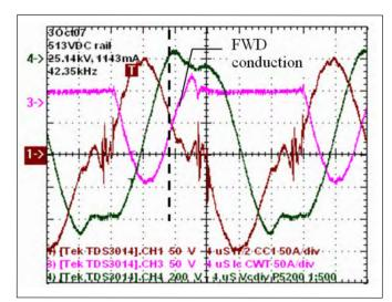
Fig. 4. Nominal line. P=28.7kW. trace 1 – primary winding current (halved); trace 3 – collector current (halved); trace 4 – voltage across resonant capacitors. FWD conducts to the right of dotted line.
