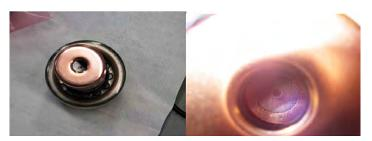
Figures 10, 11: Focal spot damage caused by inadequate anode cooling and thermo-mechanical stress
