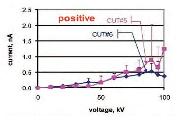
Figure 7. CUT#5, CUT#6. Leakage current at positive polarity.
