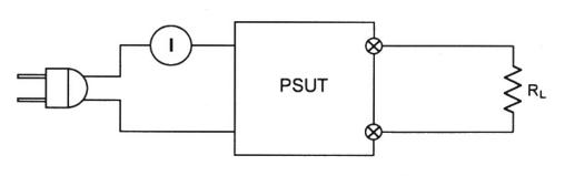
Figure 11. AC Input Current Measurement
