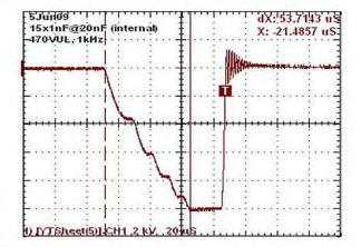
Fig. 18. 33-nF capacitor assembly under test. Charge time is 53  $\mu$ s.
