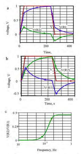
Fig. 3. Solution for equivalent circuit Fig. 2 for parameters as defined for Fig. 1. Layers' thickness  $d_1 = d_2 = 0.01 \text{ m}$ ,  $\varepsilon_1 = 2.3 \varepsilon_0$ ,  $\varepsilon_2 = 5 \varepsilon_0$ ;  $a_-\gamma_1 = 10^{-15} \Omega^{-1} \text{m}^{-1}$ ,  $\gamma_2 = 10^{-12} \Omega^{-1} \text{m}^{-1}$ ,  $b_-\gamma_1 = 10^{-12} \Omega^{-1} \text{m}^{-1}$ ,  $\gamma_2 = 10^{-15} \Omega^{-1} \text{m}^{-1}$ ,  $\gamma_2 = 10^{-12} \Omega^{-1} \text{m}^{-1}$ .
