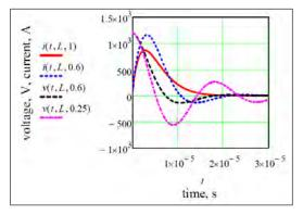
Fig. 2. Current and voltage waveforms for L=1.5 $\mu$ H; r values (in SI) as indicated in variables' legends. r=1 $\Omega$  corresponds to critically damped discharge.
