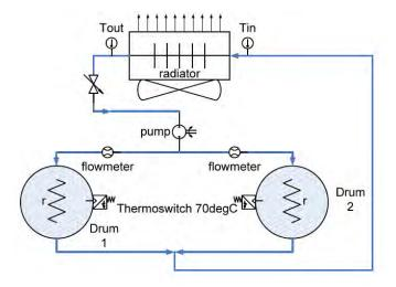
Fig. 7. Kinematic diagram of cooling system.
