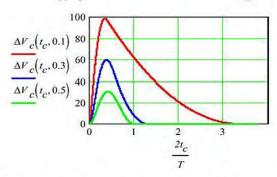
Fig. 27. Load voltage increment dependence on EOC timing  $t_c$  for  $V_{\rm r} = 550$  V. Compare to Fig. 24.
