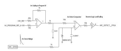
Figure 2b: Example of an Arc Detect to Scaling kV circuit in an X-Ray generator
