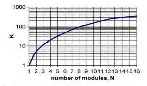
Fig. 2. Ripple suppression factor.
