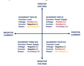
Output current and voltage are shown on the respective horizontal and vertical axis and four operational quadrants are created.
