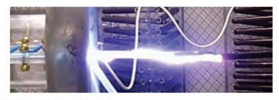
Figure 10. CUT#5. Photo of flashover. Positive polarity.
